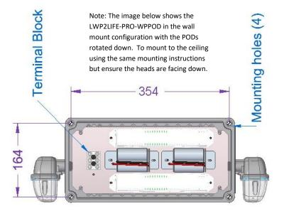
Note: When rotating the PODs in WM position ensure the PODs are level with the bottom of the main enclosure.
